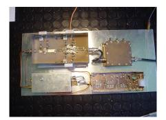
On the right bottom the oscillator and multiplier, output about 15 mW on 1296.919 Mc.
